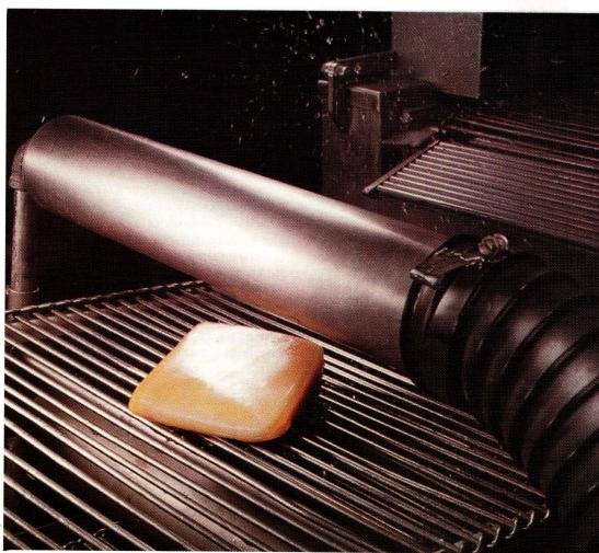
Previously, Family Fresh Pack dried wet packages of cheese manually, top. In April, the cutter and packager of cheese installed a high-velocity centrifugal blower that literally blows water droplets off the pack, thereby increasing production and deploying labor more effectively, above.
