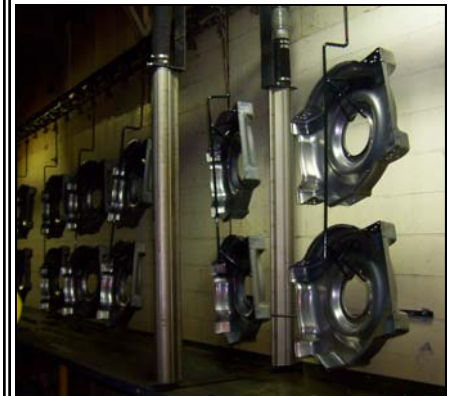
(2) 60” side knives providing final blow-off prior to painting
