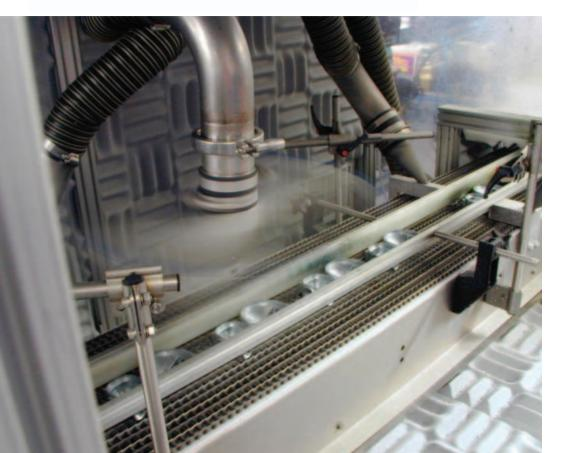
After the regulators are run through this process, they must be thoroughly dried, because any moisture left in the orifices after the regulators are assembled could lead to false gas flow rate readings. Further, the drying mechanism has to be sufficiently gentle to remove the moisture without damaging the regulators, as any surface abrasion on the gasket areas of the castings could produce failures during the pressure check.
