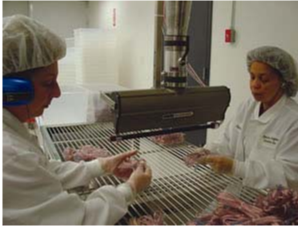
Medical cords are manually passed under the knives for static neutralization
