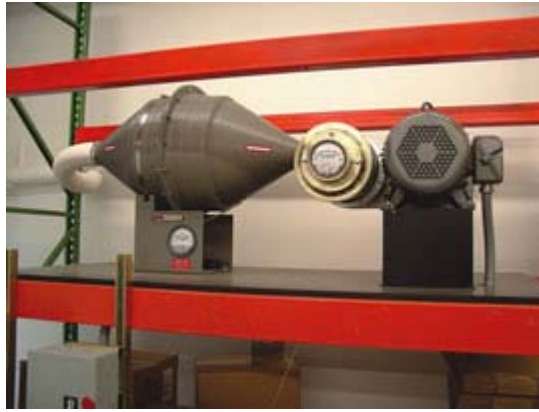
HEPA filtration directly coupled to a 20Hp centrifugal sonic blower system. Blower was mounted outside of the CleanRoom, as not to contaminate.
