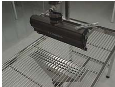
18" middle inlet air knife with ionizing bar and vacuum collection system located directly below ionized air stream
