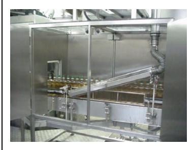
The knives were also installed with Sonic's Quick-Release brackets that allow the customer quick changes without the use of tools. Consequently, the system inserted itself into the existing production-line seamlessly without providing extra installation. For the customer the installed Sonic 150 Air System is efficient and economic.
